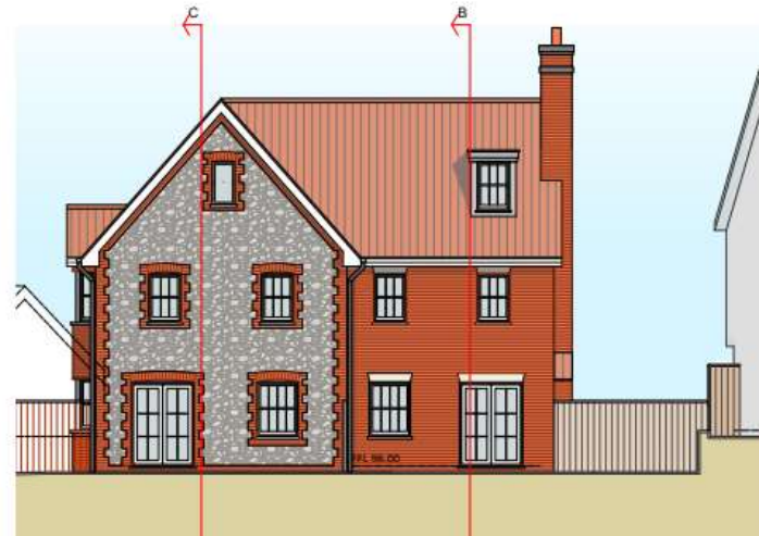
ELEVATION 3 - SOUTH FACING 1:50
